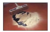
Completely cover the spill with Spillhound using the brush head, lightly press the Spillhound into the spill with a stippling action
